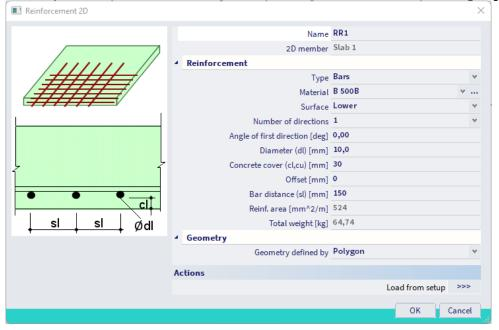
Then you can draw an area in which you want this reinforcement to be taken into account. For this example we define the above reinforcement on the largest span of the slab:
